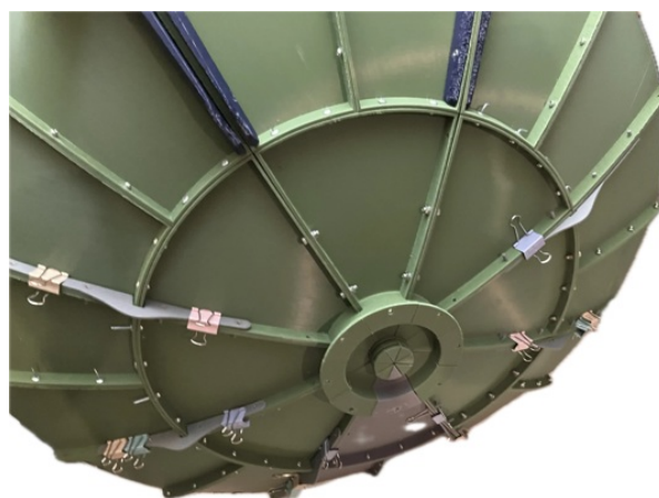
Rear structure and radial support ribs.
