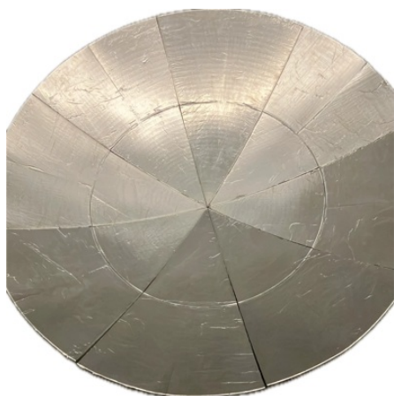
Front of the segmented reflector.
