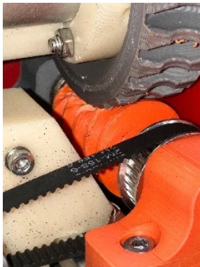
Damaged PLA worm gear documented after testing.
