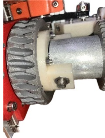
A bolted connection introduced to reduce slipping.
